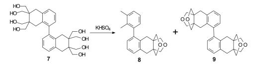
Mono-propellane **8** is probably produced in the first step by the retro *Diels-Alder* reaction [12] of **9** according to the scheme given below.
